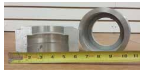
Figure 4. Photo of the mockup used as a proof of concept for the aluminum actuator.
