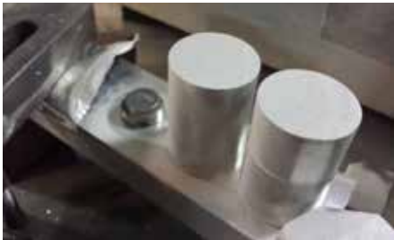
Figure 6. Photo of the ASTM C633 bond test specimens deposited for proof of concept testing.
