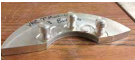
Figure 7. Photo of the simulated C633 bond testing on the mockup.
