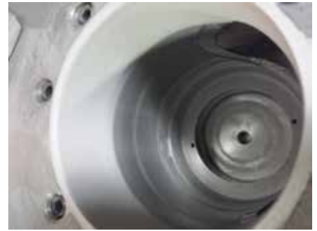
Figure 9. Photo of the aluminum actuator internal bore repair.
